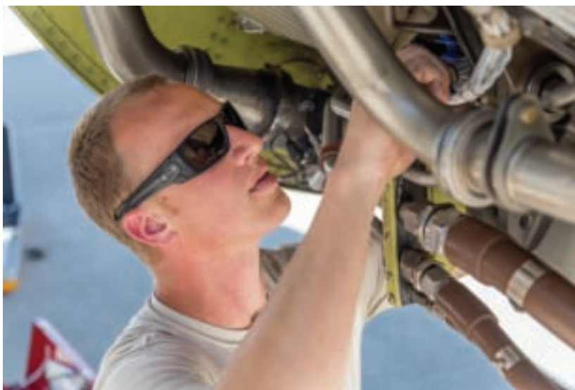
Tech. Sgt. Kyle Perry from the Guidance and Control Shop performs a wire-harness repair on a jet engine.
