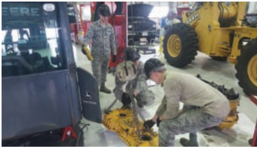
Staff Sgt. Daniel Soto, Senior Airman Reno Rivers and Senior Airman Parker Sheffield, vehicle mechanics assigned to the 151st LRS, use a three-ton crane to fix a transmission for a John Deere loader.
